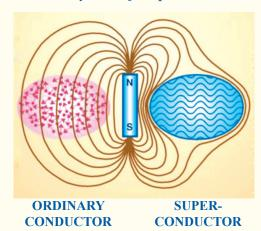
In an ordinary electrical conductor (left), incoherent disordered electrons allow penetration by an external magnetic field. In a superconductor (right), coherent collective functioning of the electrons spontaneously repels an external magnetic field, and maintains its impenetrable status.
